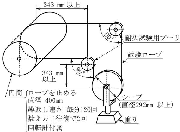
Fig.1 Model of durability experiment device provided by JIS<sup>1</sup>
