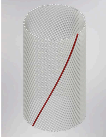
Fig. 3 Muscle layout of cylindrical mechanism is helical. A red string is a thin McKibben muscle.
