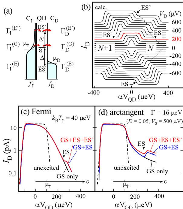
FIG. S 4. (a) Energy diagram of transport through a QD. ES and ES' are first excited states of  $N$ - and  $(N+1)$ -electron QDs, respectively. (b) Calculated QD current  $I_D$  as a function of electrostatic potential  $\alpha V_{QD}$  at various  $V_D$ . (c) and (d)  $I_D$  at  $V_D = 200 \mu\text{V}$  with a heated Fermi distribution function for (c) and an arctangent function for (d) in  $C_{\uparrow}$ .
