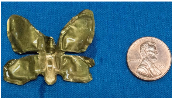
Fig. 10 Butterfly robot (butterfly shaped IPMC actuator)
