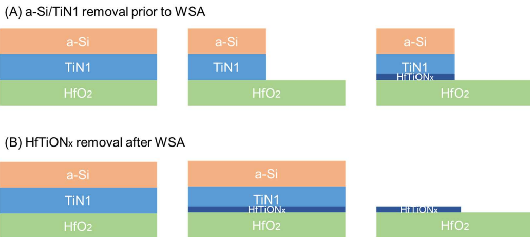
Figure 2-13 Schematics for possible multi- V_T integration using eWF control technique discussed in this work. (A) a-Si/TiN1 removal prior to WSA, (B) HfTiON_x removal after WSA.
