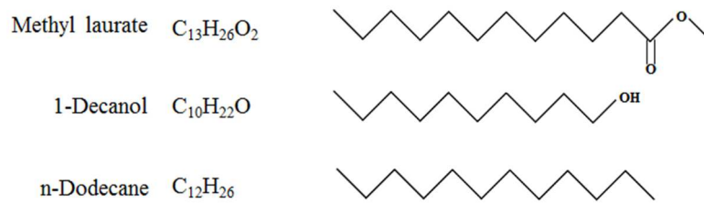
Figure 4- 1 Chemical structure of main fuel used in this chapter for a comparison study.
