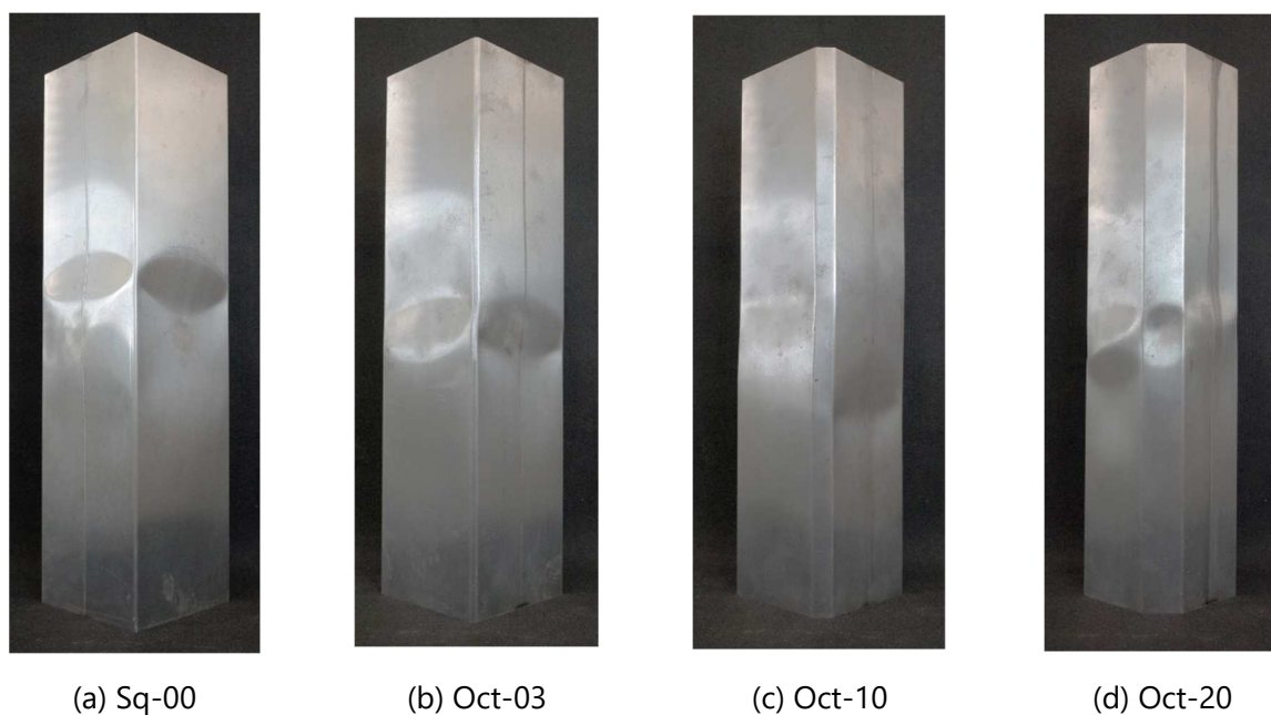
Fig. 4.A Collapse mode of each specimen
