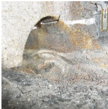
(a) Crack at the weld access hole
