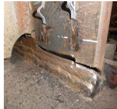
(c) Propagation of cracks
