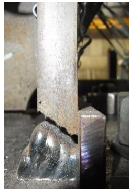
(b) Crack at the weld toe
