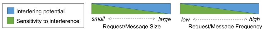
Figure 5.12: An illustration of the interfering potential and interference sensitivity of communication sizes and frequencies. Note: This figure illustrates general trends and not precise performance results. The changes in potential and sensitivity are not expected to be linearly proportional.
