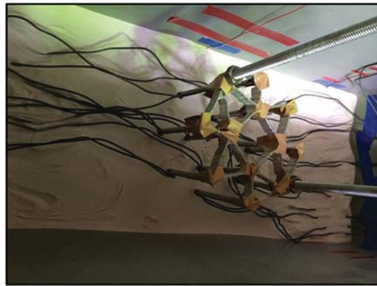
(b) Piles fixed at box center during sand pouring.
