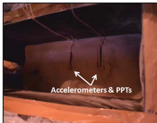
(c) Model ground sensors during sand pouring.
