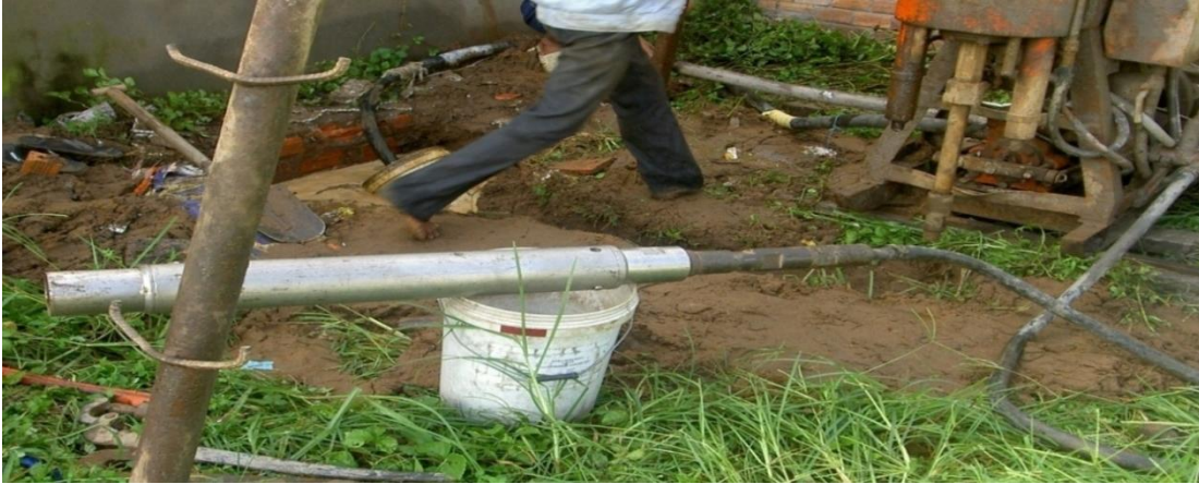
(a) Tube sampler was assembled the fixed piston and joint, and then checking move of piston.
