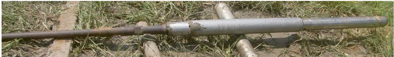
(b) Tube sampler and fixed piston was assembled rod.
