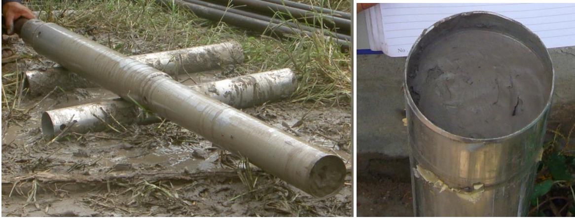
(d) Soil sample in tube sampler was taken out of the borehole and was cleaned at Vinhlong site.
