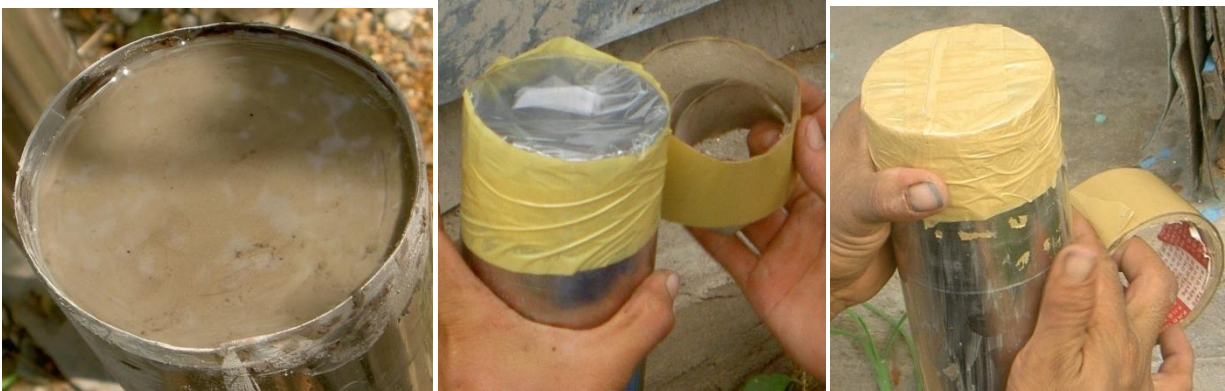
(e) Soil sample in tube sampler was covered by paraffin, plastic and sticking-plaster.
