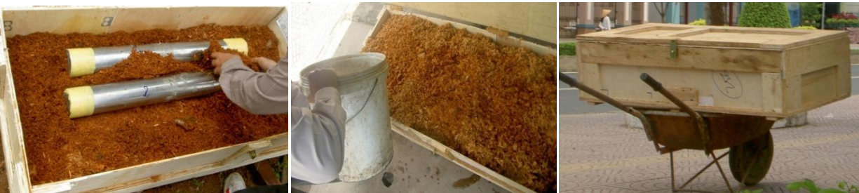
(f) Samplers arranged and covered by soft material with water, sampler-barrel was carried.
