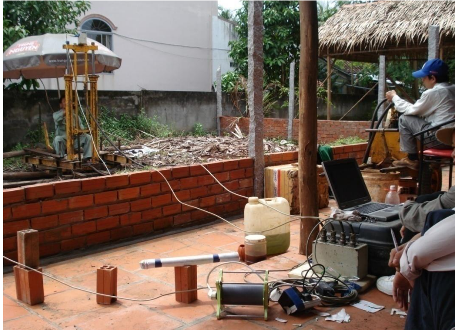
Fig. 3.7. CPTU test was conducting at Vinhlong site in Vinhlong province MRD.
