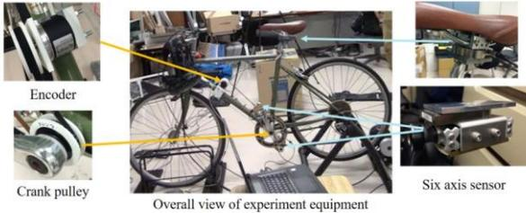
Fig. 6 Overall view of experiment equipment and sensors
