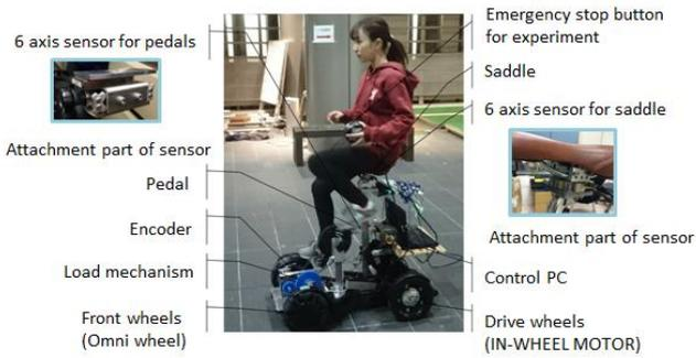
Fig. 2. The prototype of new concept vehicle
