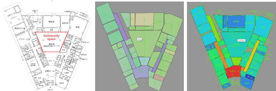
Fig. 5.22 Original common space floor plan(left), and spatial mean depth(middle) and integration result(right) (Source: created by author)
