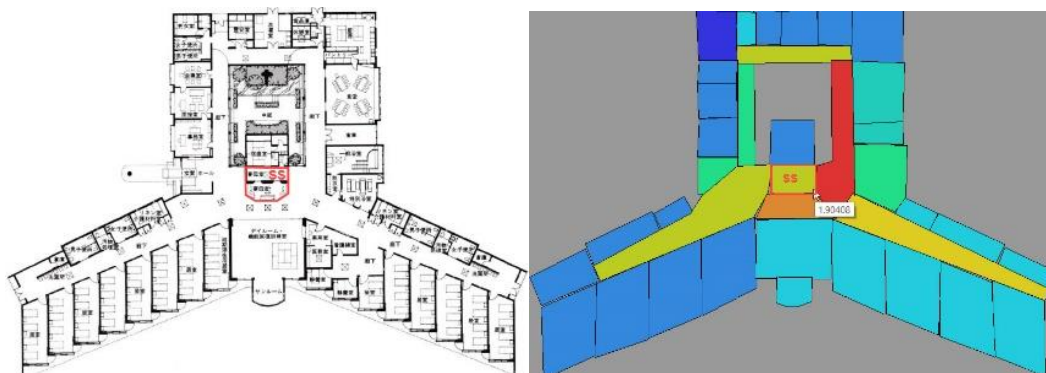
Fig. 3.11 SST in a classical large-scale care type nursing home (Source: created by author, NHID:11)
