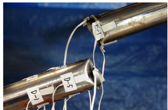
(f) Brace gross section fracture (150%-1st)
