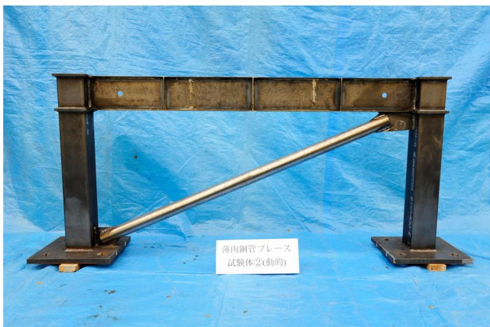
Photo 2.3.1 Specimen before shake table testing
