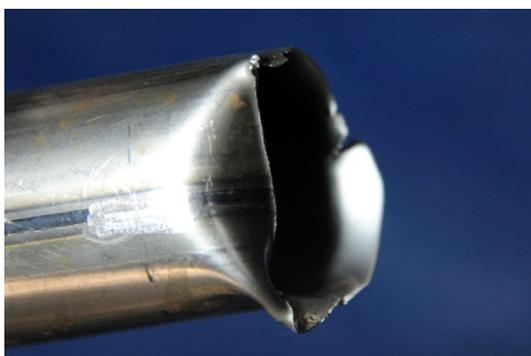
(g) Fracture section (after testing, left side)
