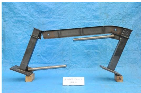
(e) Collapsed specimen after testing
