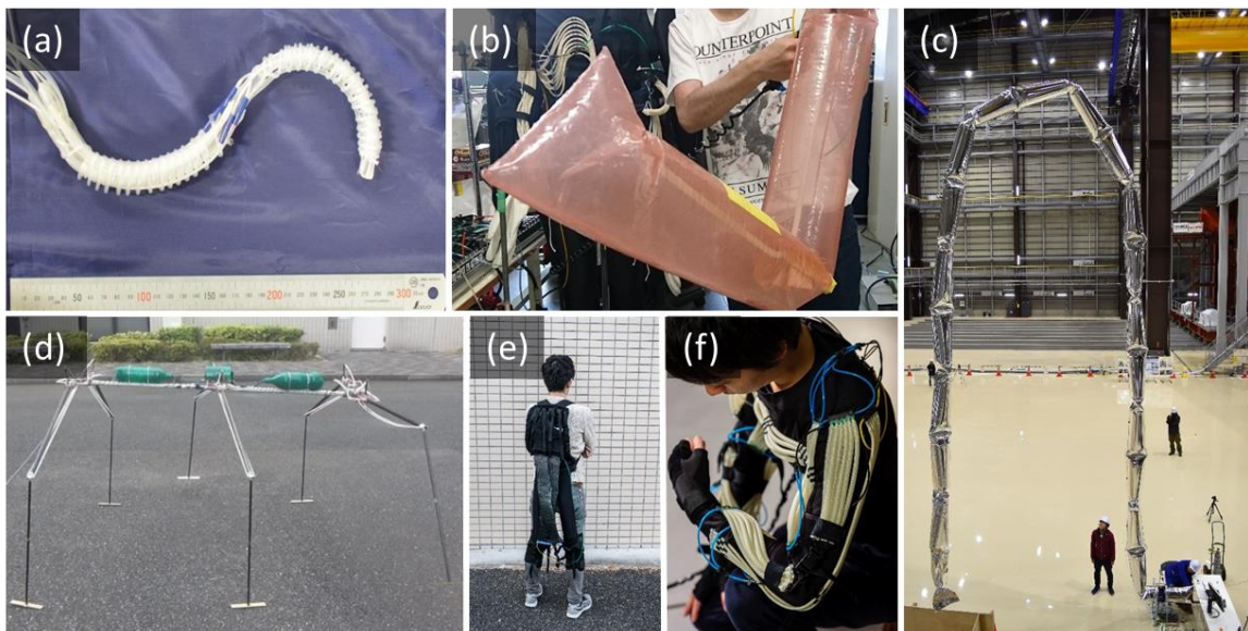
Figure 1.3 Application of thin McKibben muscles. (a) Biomimetic octopus arm [119]. (b) Exoskeleton inflatable robotic Arm [120]. (c) 20 m balloon Giacometti arm [123]. (d) Long-legged hexapod Giacometti robot [124]. (e) Assist suit for lower limb. (f) Assist suit for upper limb.
