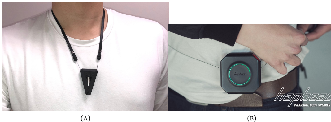
FIGURE 6.1: The current and last versions of the Hapbeat wearable haptic interface, which may be an ideal haptic device for the next revision of the Haptic Music Player [©HapBeat].
