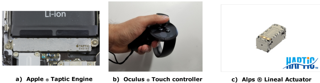
FIGURE 1.1: This figure shows diverse haptic actuators used in modern handheld devices. a) The haptic actuator used in Apple cell-phones, where the amplitude of the signal can be controlled [45]. b) Oculus touch controller, equipped with haptic actuators with a refresh rate of 320Hz and a frequency range of 0~160Hz. c) a state of the art lineal actuator with a wide frequency range of 0~450Hz. [11]
