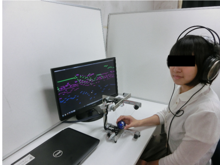
FIGURE 1.2: This figure shows the complete Haptic Music Player environment. The environment plays a MIDI song, along the music, while the user can see a graphical representation of the song melody and also can feel the vibration of an specific instrument of the song. Our hypothesis is that, the complete system helps the users to focus their listening attention to have a closer and deeper understanding of the music.
