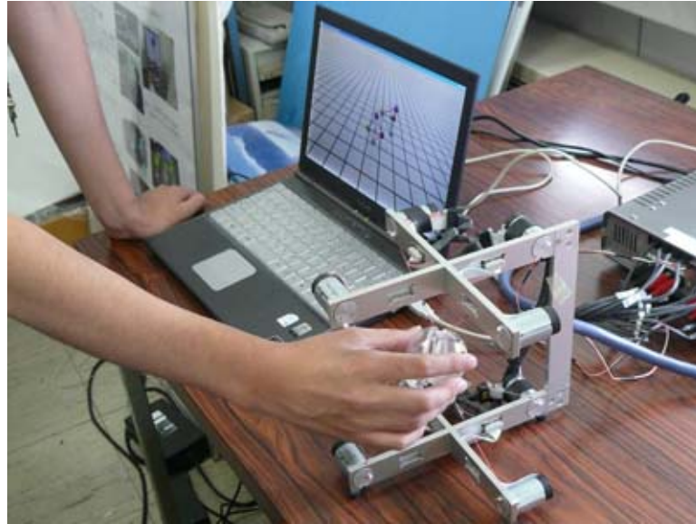
FIGURE 5.9: This figure shows SPIDAR-G6 being used for a 3D virtual reality application. We implemented the Haptic Music Player in SPIDAR-G6 mostly because the performed psychophysical experiments required small latency between the audio and haptic signals. By using SPIDAR-G6 drivers we could achieve a delay time of \pm 2 ms. © [2002] IEEE [29].
