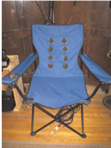
FIGURE 2.1: shows the haptic interface proposed by Karam, composed of 8 speakers on the back of the chair. Uses a haptic metaphor to display the signal [27] © [2009] IEEE.
