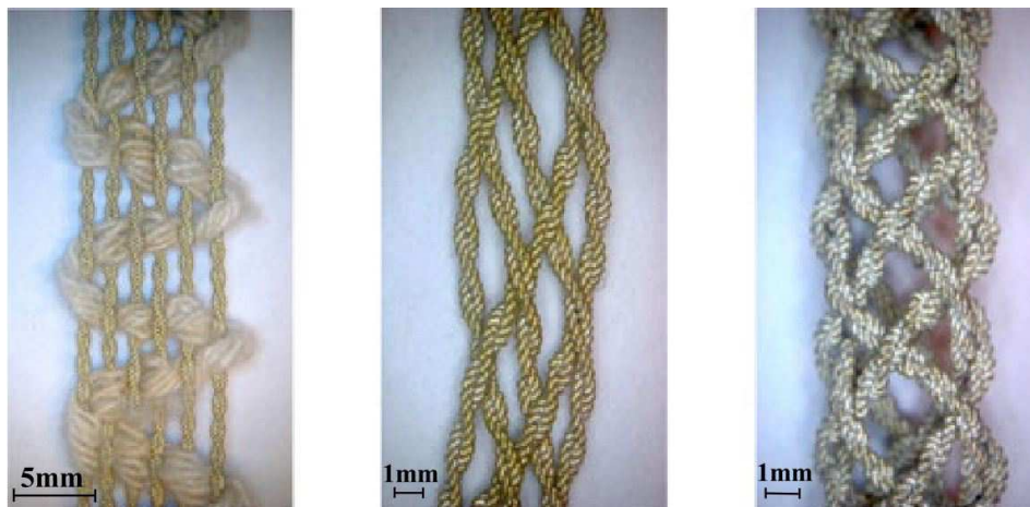
Figure 1.9 Active textile using super coiled polymers, Simeonov et al.(2018) [26].
