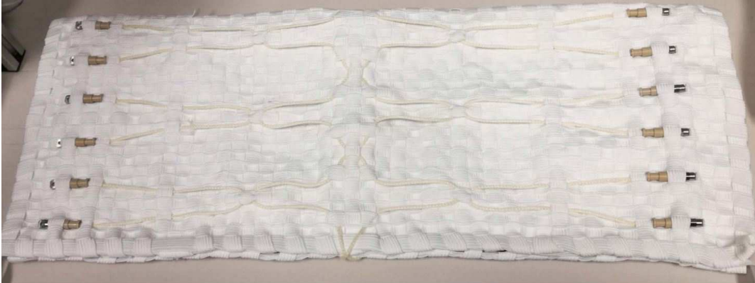
Figure 1.10 Active textile using thin McKibben muscles, Funabora(2018) [28].
