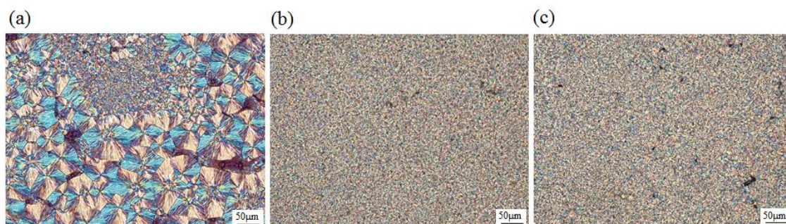
Fig. 7: Polarization-microscope images of pellets and powder obtained at RT after temperature crystallization at 190 °C for 60 min: (a) pellets and (b) powder (c) powder with 0.1-wt% addition of fumed silica.
