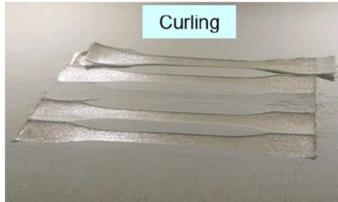
Fig. 8: Problems observed during SLS processing: “curling” [19]
