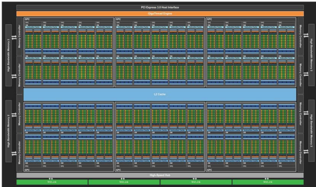
FIGURE 2.1: Architecture of NVIDIA GP100 (Source: NVIDIA Tesla P100 Whitepaper [40])
