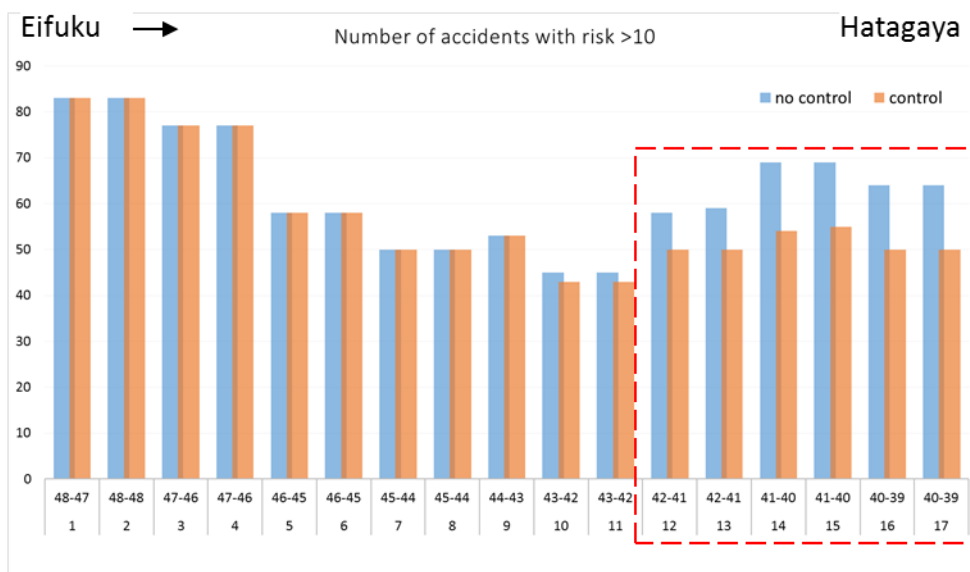
Figure 5. 17 Comparison of NER \geq 10 with and without VSL Control (QL) (cell 9 to 17)
