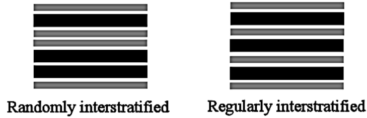
Fig. 1. 12 Types of mixed-layering (modified from Nadeau et al, 1984) [43].
