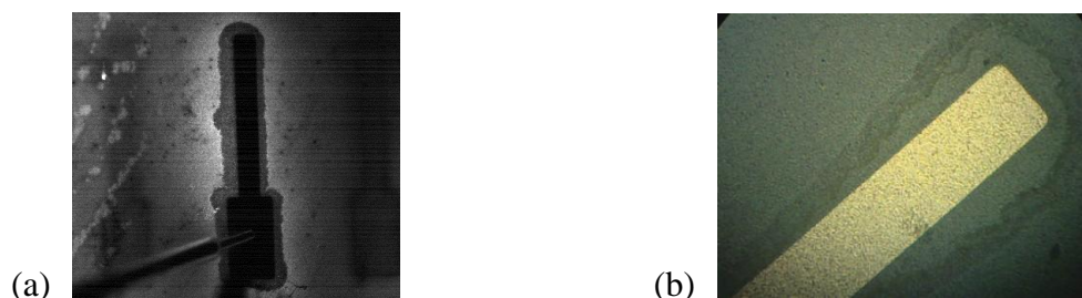
Figure 4.12: The defects after applying voltage (a) under measurement (b) optical image after measurement
