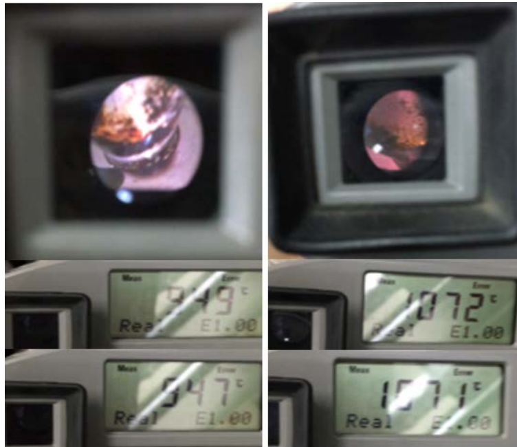
Fig. 2-9 Temperature measurement at the location of the upper region for (a) Ar plasma and (b) Ar/H 2 plasma by the infrared thermometer.
