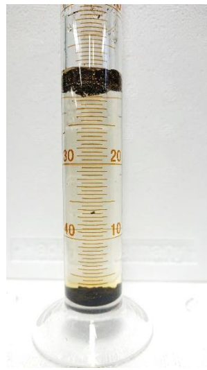
Figure 2.14 Different of material density shown by floating aluminum and submerging chars in the water column
