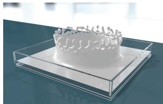
Fig.2.63: The predicted time evolution of gas-liquid interface, obtained at 297 \times 297 \times 108 meshes for the milk crown simulation
