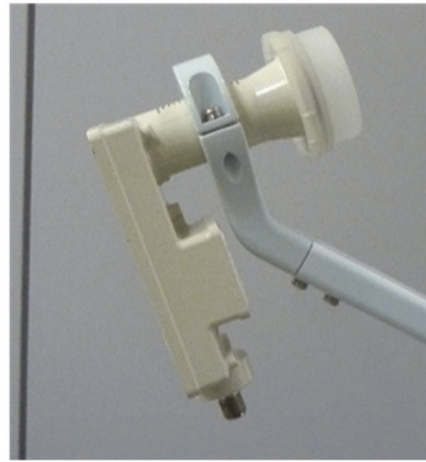
(b) Feed horn and LNB.
