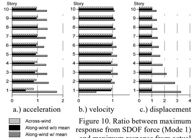
Figure 10. Ratio between maximum response from SDOF force (Mode 1) and maximum response from actual wind force
