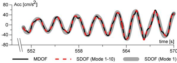
Figure 4. Comparison of acceleration response from MDOF and SDOF analysis (roof level)
