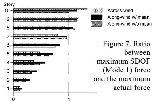
Figure 7. Ratio between maximum SDOF (Mode 1) force and the maximum actual force
