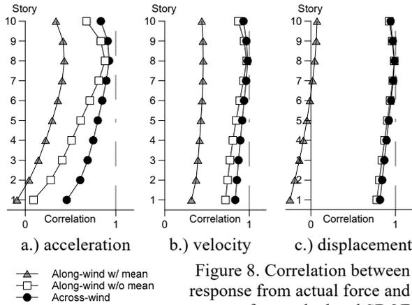
Figure 8. Correlation between response from actual force and response from calculated SDOF (Mode 1) force
