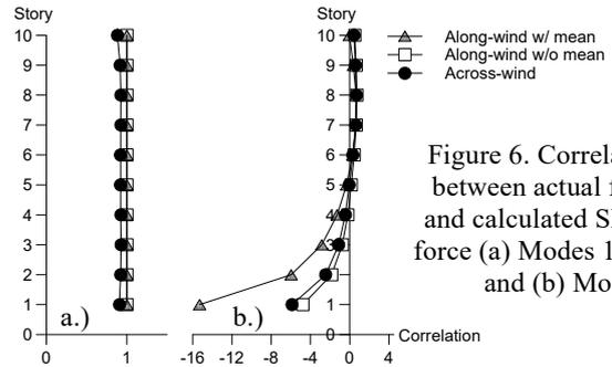
Figure 6. Correlation between actual force and calculated SDOF force (a) Modes 1~10, and (b) Mode 1.
