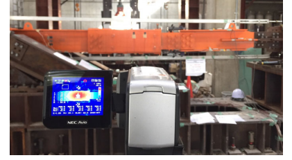
Figure 3. Thermal imaging device capturing the damper temperature.
