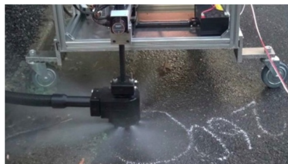
Figure 15 The robot during the decontamination experiment - Around the Nozzle. Substantial water leakage is shown, which was because the positioning precision was degraded by sensor jamming due to the water leakage.
