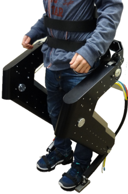
Fig. 1: The pneumatic lower limb exoskeleton
