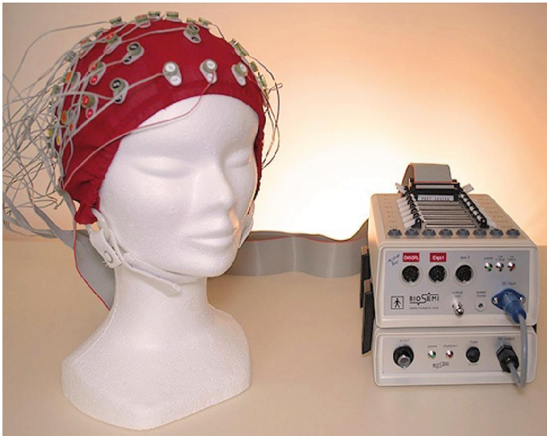
Figure 2.13: Bio-semi EEG acquisition system [5]
