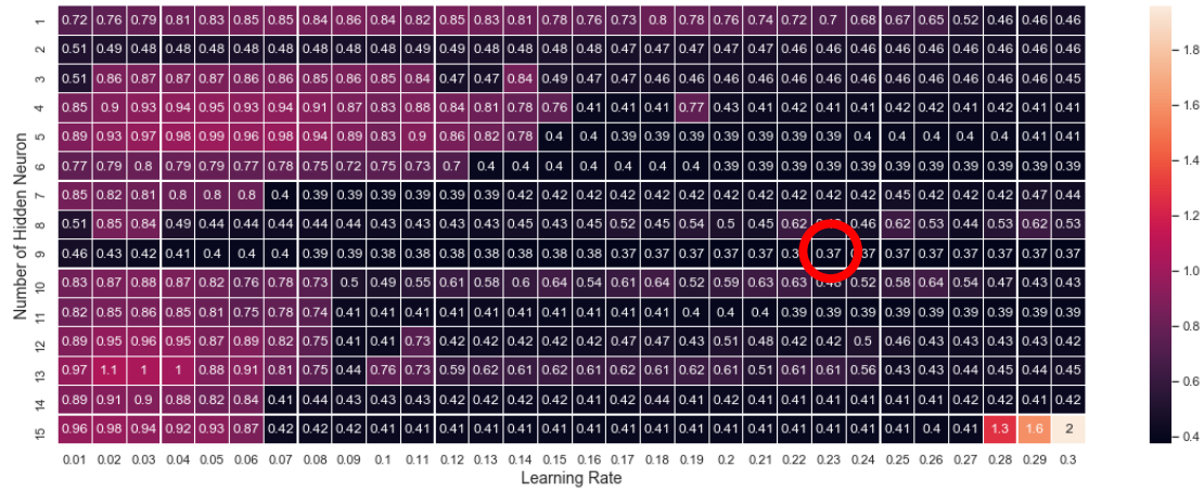
Figure 4. 4 Plot of MSE of ANN from several combination of hidden neuron and learning rate for fibrinogen adsorption prediction of multi-lab data
