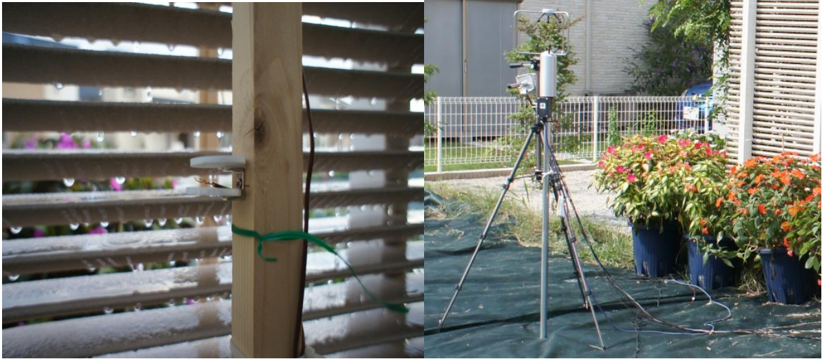
(a) Thermocouple with shield (b) T_{amb} , Solar radiation, RH, WS_{out} , WD_{out}
