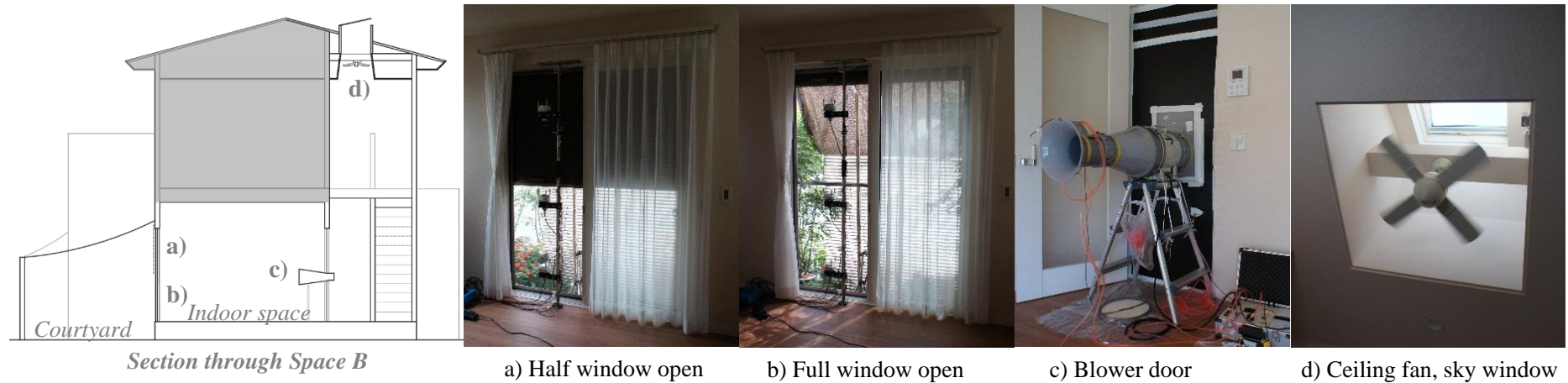
Figure 2.4. Location and photos of ventilation settings.
