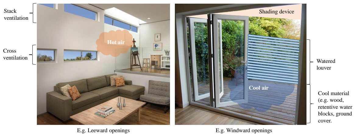
Figure 6.1 Example of sizes for windward and leeward opening for generating cool microclimates inside buildings
