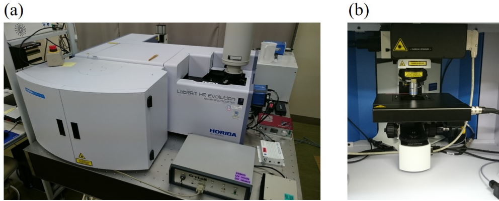
Fig. 4.7: (a) Raman spectrometer and (b) its inside.
