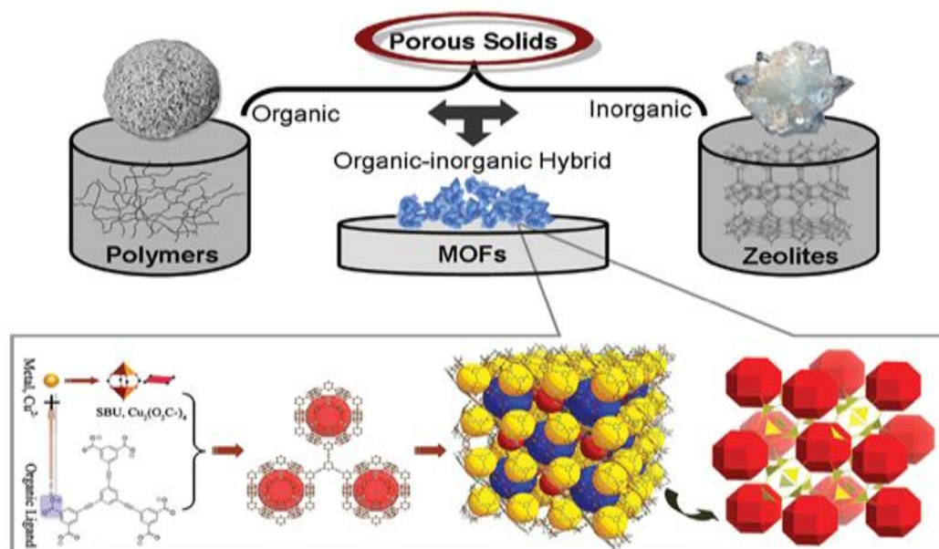
Fig. 2.3 Schematic diagram of classification porous solids and construction procedures of MOFs
