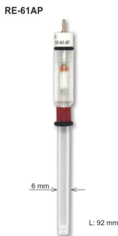
Figure 3.4: Commercial Hg/HgO reference electrode for alkaline solution. Internal solution is 3 M NaOH with E^0 = 241 mV vs RHE (25 °C). RHE = Reversible hydrogen electrode. Used for alkaline electrolytes. Image copyright 2001-2020 by ALS Co., Ltd
