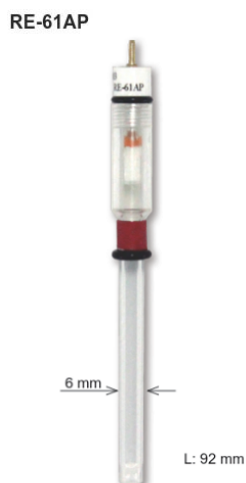
Figure 3.4: Commercial Hg/HgO reference electrode for alkaline solution. Internal solution is 3 M NaOH with E^0 = 241 mV vs RHE (25 °C). RHE = Reversible hydrogen electrode. Used for alkaline electrolytes. Image copyright 2001-2020 by ALS Co., Ltd
