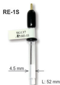
Figure 3.3: Commercial Ag/AgCl reference electrode for acidic solution. Internal solution is 3 M NaCl with E^0 = 195 mV vs RHE (25 °C). RHE = Reversible hydrogen electrode. Used for acidic electrolytes. Image copyright 2001-2020 by ALS Co., Ltd
