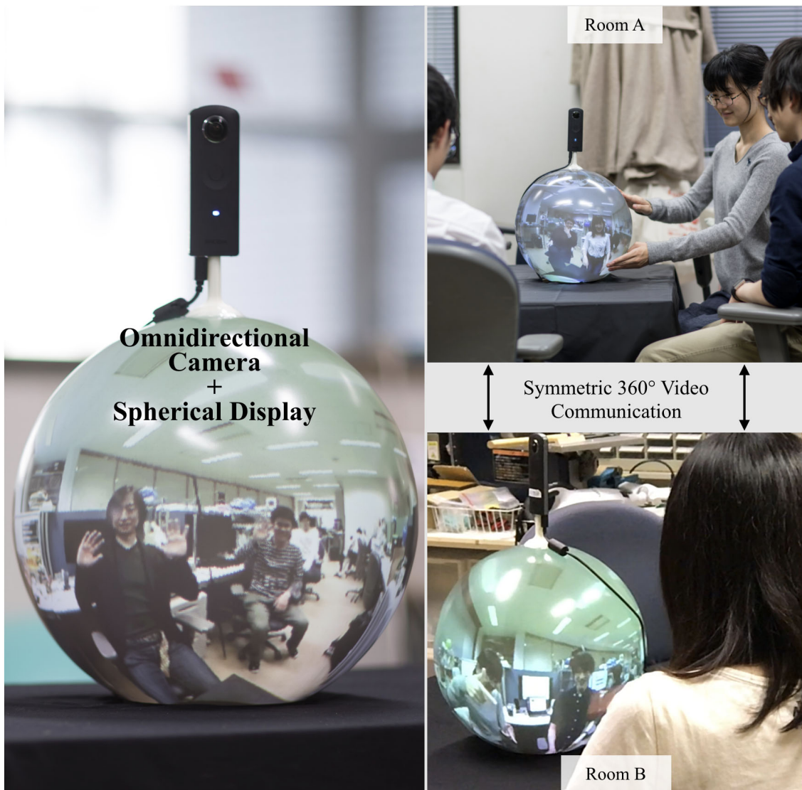
Figure 5.1: The OmniEyeball2 system which integrates an omnidirectional camera with a full spherical display (left), and its symmetric 360° panoramic video communication application (right).
