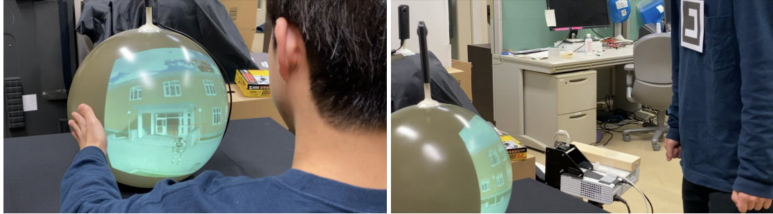
Figure 6.8: In the third-person mode, the designers can rotate or walks around the OmniEyeball in order to observe the VR space at a different direction.
