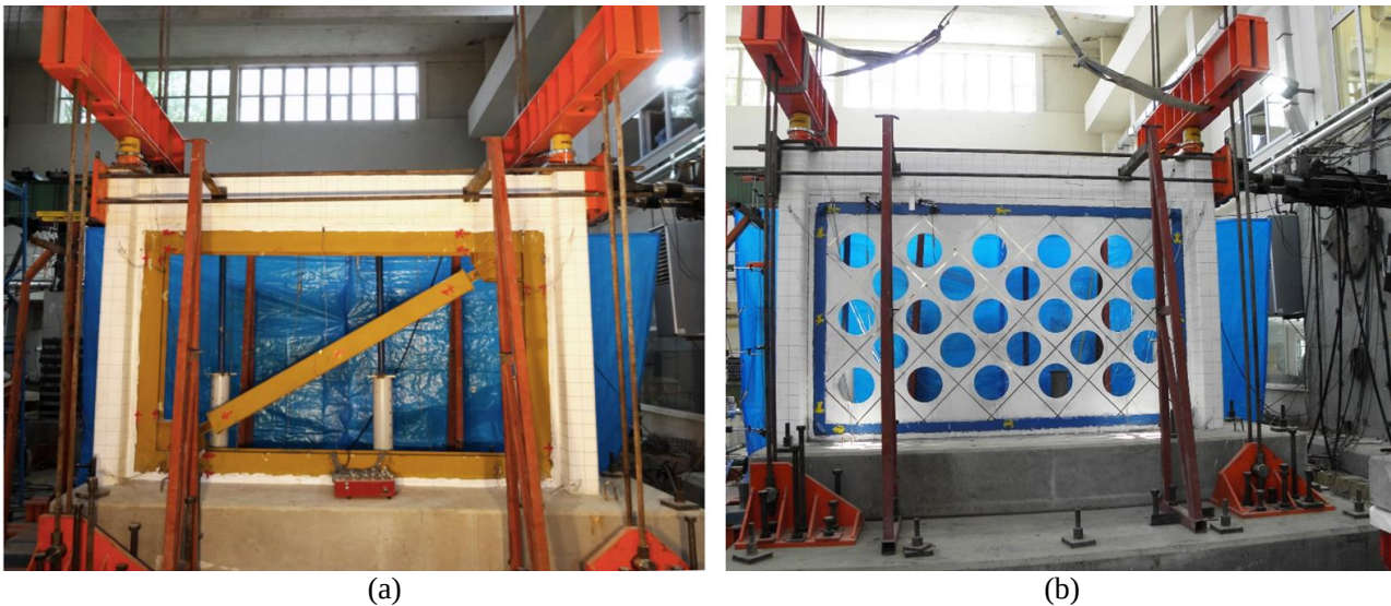
Fig. 1 - General view of (a) RSB model and (b) RSP model test set-up.
