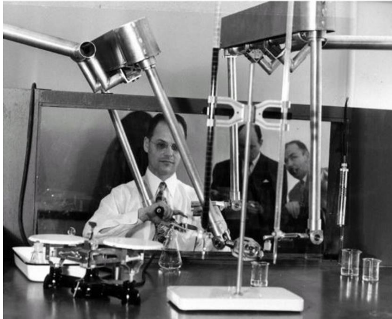
Fig. 1.1 The first master-slave manipulator “model M1” [1].
