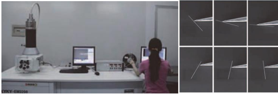
Fig. 1.4 The tele-nanomanipulation platform (left) and the appearance of moving a wire that consists of single ZnO molecules (right) [5].
