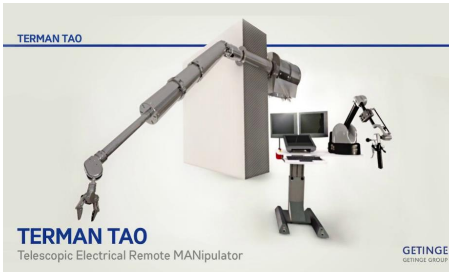
Fig. 1.2 “TERMAN TAO”, a master-slave system widely used in nuclear industries around the world [2].
