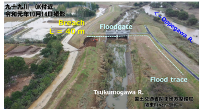
Fig. 6. Breach at 7.6 k on left levee of Opegawa River. The drone image was obtained from the database maintained by the Ministry of Land, Infrastructure, Transport and Tourism, Japan ( https://www.ktr.mlit.go.jp/bousai/index00000051.html ).
