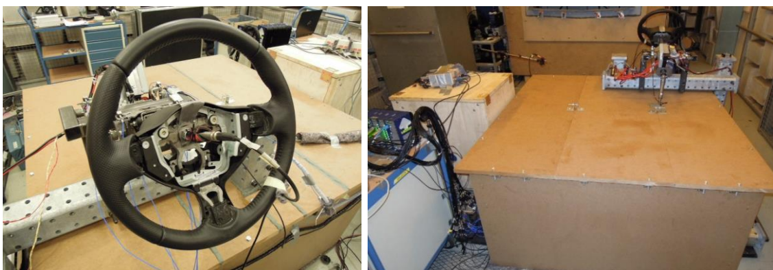
Fig. 5.9 A microphone mounted at the steering wheel center from which the airbag module has been removed and overview of the EPS component test bench encapsulated by wooden box with the steering wheel.
