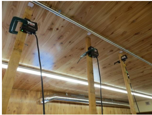
(b) 変位計設置の様子[拡大]
