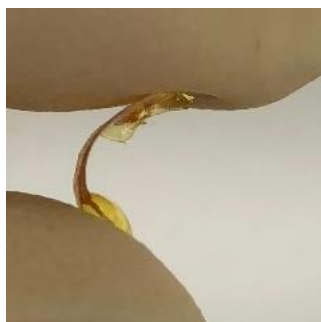
Figure 6-18. Porous polyimide film based on PAA6/PI- b -P2VP3/R1.
