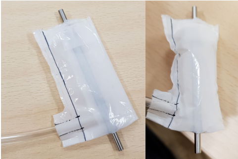
Figure 5.18: Airbag made by polyethylene sheet
