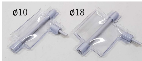
Figure 5.12: Two types of airbags made by PVC
