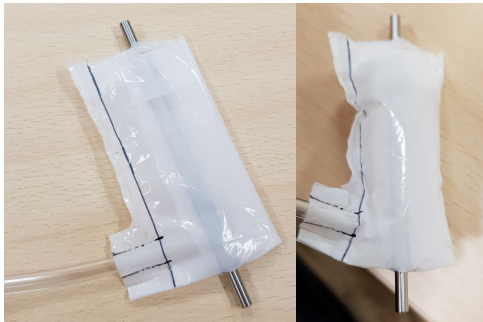
Figure 5.18: Airbag made by polyethylene sheet
