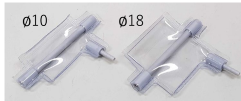
Figure 5.12: Two types of airbags made by PVC
