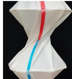
Figure 2.4: Extension limit because of collision between paper edges
