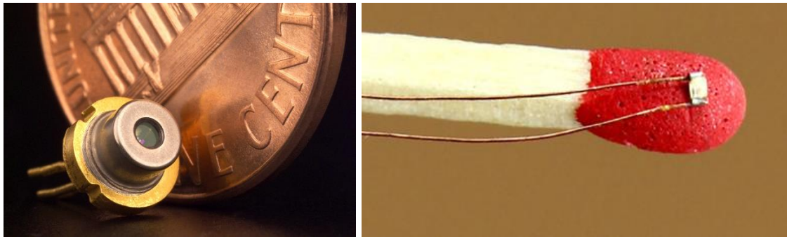
Fig. 1.20 Size of semiconductor light source (left: LD; right: LED) [114]
