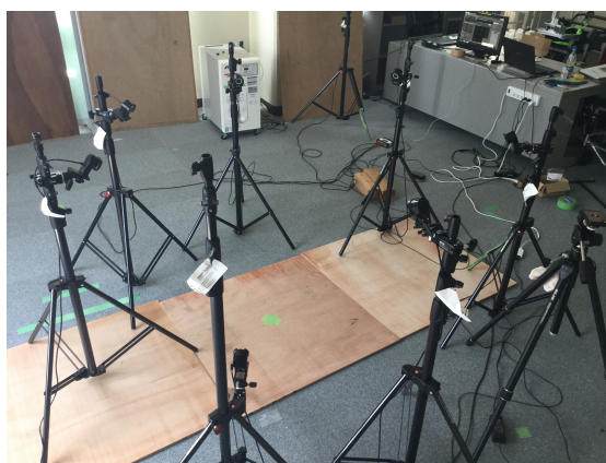
Figure 5.1: Measurement environment of motion capture system (adapted from [65]).
