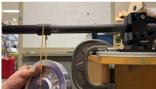
Fig.3 Fix CFRP pipe to OTA's output axis
