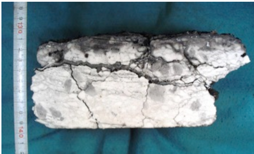
Fig. 1-18. An example of structural spalling by slag infiltration. The material is an Al 2 O 3 -MgO low cement castable used in a steel ladle.
